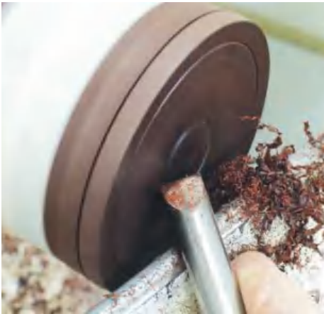
STEP 31. Add some decorative grooves using the point of the skew chisel; this adds a little interest to the piece. The rosewood is very dense so a good finish can be achieved straight off the tool
